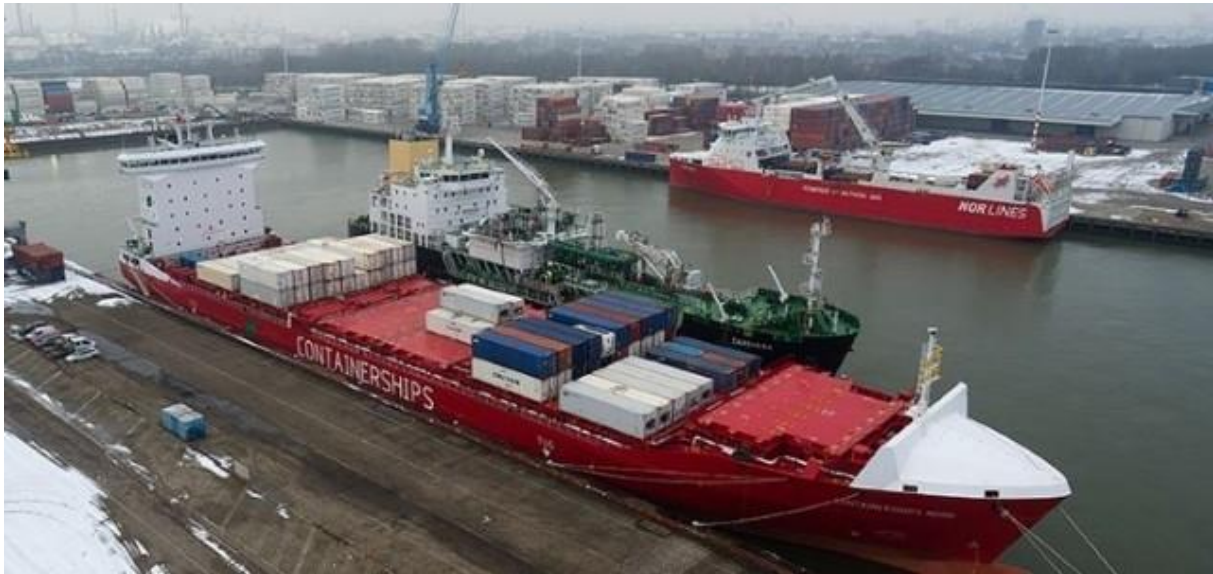
Containerships Nord was refuelled by Shell's LNG bunker vessel Cardissa in the Port of Rotterdam. Foto:
